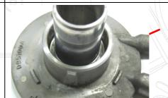
White coloured seal at bottom of CSC bore
