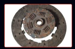
Clutch has failed at the segment necks due to misalignment between engine and transmission.
