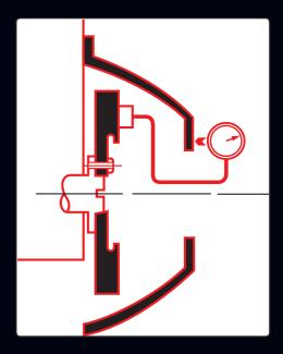
STEP 2 With indicator still mounted to flywheel ensure rear surface of housing is square.
