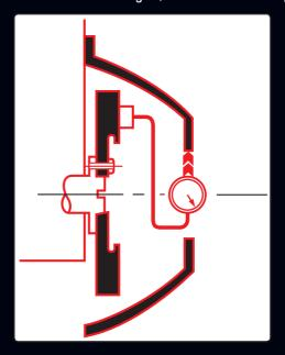
STEP 1 Mount indicator to flywheel and determine concentricity of bell housing bore to centre line of crank rotation. SPECIFICATION: 0.15mm max. T.I.R.
