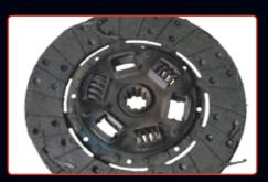
Incorrect cover assembly or incorrect clutch release mechanism adjustment or driver abuse.
