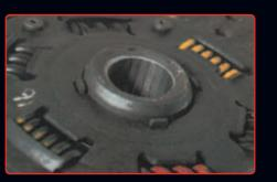
Result of incorrect clutch driven plate for the application.
