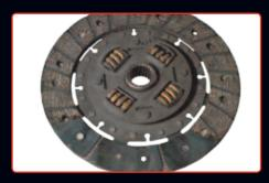
Burst facing usually caused by driver abuse, such as severe down changing through gears, ie 5th to 2nd at excessive road speed.
