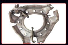
Centrifugal failure of 11 inch clutch due to non-standard installation. Possibly in lieu of twin plate.
