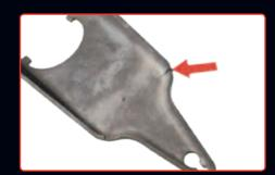
Unable to achieve clutch release. Incorrect cable adjustment caused by cracked release fork.
